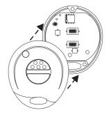
Separate the shell halves taking care not to damage the internal circuit.
